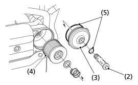
(2) oil filter bolt(3) oil filter cover
