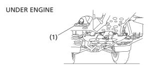
(1) engine oil drain bolt
