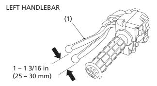
(1) rear brake lever/parking brake lever
