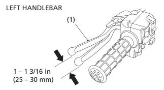
(1) rear brake lever/parking brake lever
