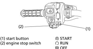
The start button (1) is used for starting the engine. Pushing the button in starts the engine. See *Starting Procedure*, page 68.
