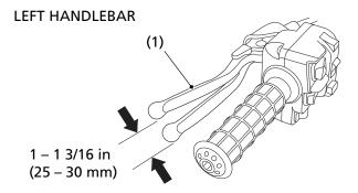
(1) rear brake lever/parking brake lever
