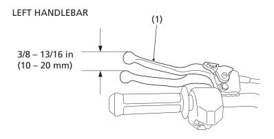
(1) rear brake lever/parking brake lever
