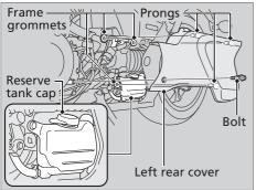
5. Remove the reserve tank cap and add fluid while monitoring the coolant level.
