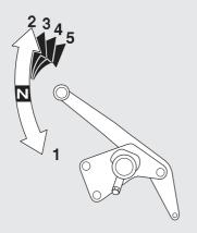
If you put the motorcycle in gear with the side stand down, the engine will shut off.
