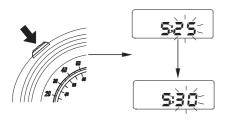
7. To end the adjustment, push and hold the odometer/tripmeter/digital clock select and reset button for more than 2 seconds or turn the ignition switch OFF. The display will stop flashing automatically and the adjustment will be cancelled if the button is not pressed for about 30 seconds.
