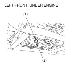
(1) engine oil drain bolt(2) sealing washer
