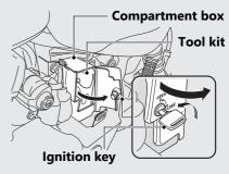
Insert the ignition key and turn it counterclockwise to unlock.
