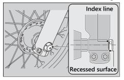
4. Tighten the left axle pinch bolts.
