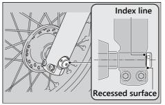
4. Tighten the left axle pinch bolts.
