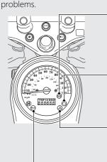
(S) ABS (Anti-lock Brake System) indicator VT750CS
