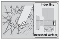
4. Tighten the left axle pinch bolts.
