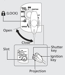
The shutter will automatically close when you remove the ignition key at the (LOCK) position.
