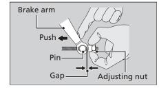
After adjustment, confirm the freeplay of the brake lever.
