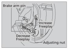
**2.** Apply the brake several times and check for free wheel rotation after the brake lever is released.
