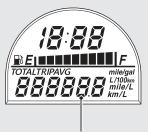
**Odometer [TOTAL] & Tripmeter [TRIP] & Average fuel mileage meter [AVG]** Mode switch selects the odometer, tripmeter and average fuel mileage.
