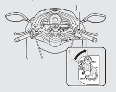
Press the start button with the throttle completely closed. Release the start button as soon as the engine starts.
