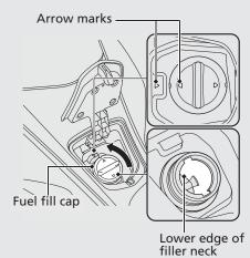
Do not fill with fuel above the lower edge of the filler neck.
