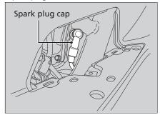
**8.** Install the new spark plug. With the plug washer attached, thread the spark plug in by hand to prevent cross-threading.
