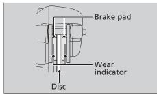
**1.** Inspect the brake pads from underneath the brake caliper.
