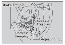
Apply the brake several times and check for free wheel rotation after the brake lever is released. **3.** Push the brake arm to confirm that there is a gap between the rear brake adjusting nut and brake arm pin.
