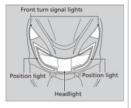
The headlight/front turn signal lights/position lights use several LEDs.
