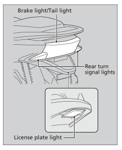
The brake light/tail light/rear turn signal lights/license plate light use several LEDs. If there is a LED which is not turned on, see your dealer for this servicing.
