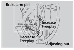
Apply the brake several times and check for free wheel rotation after the brake lever is released. **3.** Push the brake arm to confirm that there is a gap between the rear brake adjusting nut and brake arm pin.
