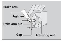
After adjustment, confirm the freeplay of the brake lever.
