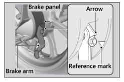
When the brake is applied, an arrow attached to the brake arm moves toward a reference mark on the brake panel. If the arrow aligns with the reference mark on full application of the brake, the brake shoes must be replaced. See your dealer for this service.
