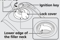
Do not fill with fuel above the lower edge of the filler neck.
