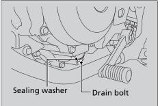
**6.** Install a new sealing washer onto the drain bolt. Tighten the drain bolt.
