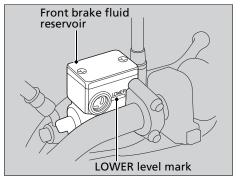
If the brake fluid level in the reservoir is below the LOWER level mark or the brake lever freeplay becomes excessive, inspect the brake pads for wear. If the brake pads are not worn, you most likely have a leak. Have your motorcycle inspected by your dealer.
