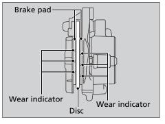
**1.** Inspect the brake pads from in front of the brake caliper.
