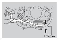
Make sure the brake rod, brake arm, spring and fastener are in good condition.
