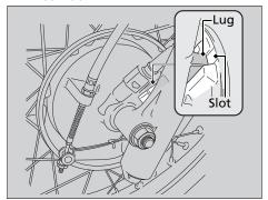
**3.** Make sure that the lug on the left fork leg is located in the slot of the brake panel.
