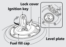
Do not fill with fuel above the level plate. **Fuel type:** Unleaded gasoline only **Recommended fuel octane number:** Pump Octane Number (PON) 86 or higher. **Tank capacity:** 1.48 US gal (5.6 L)
