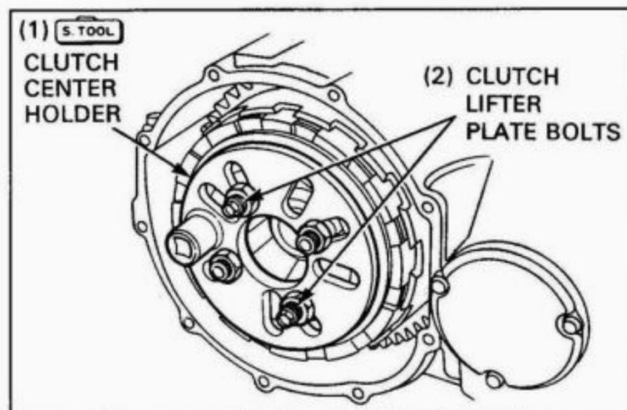
Hold the clutch center holder and remove the lock nut as shown.
