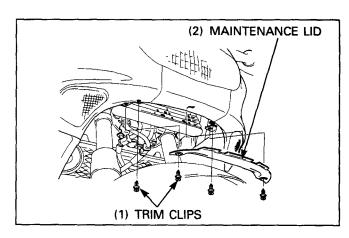
Remove the trim clips connecting the both lower fairings.
