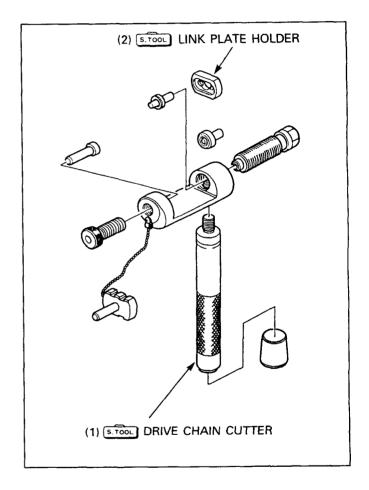
Locate the crimped pin ends of the master link from the outside of the chain and remove the link with the chain cutter.
