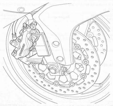
Along with these new radial-mounted front brake calipers, the new front brake system features a newly developed vertical piston layout master cylinder. This system minimizes lost motion and moves the lever pivot farther away from the end of the lever which offers high braking efficiency with excellent feel and controllability.
