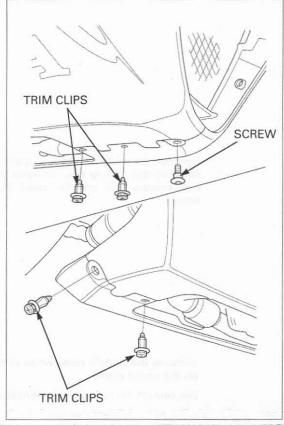
Remove the six trim clips from the inner lower cowl and inner middle cowl.
