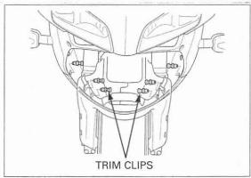
Remove the under cowl-to-middle cowl pan screws. Remove the under cowl mounting special screws and then remove the under cowls and inner lower cowl.
