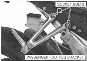
Remove the socket bolts and right footpeg bracket.
