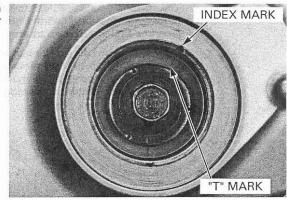
for reference in shim selection if VALVE CLEARANCE: required.
