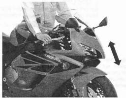
Check for worn steering stem bearings by grabbing the front fork legs and attempting to move the front fork front to back.
