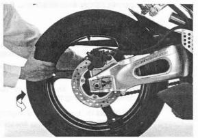
Check for worn swingarm bearings by grabbing the rear end of the swingarm and attempting to move the swingarm side to side.
