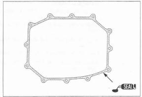
Install the oil pan onto the lower crankcase. Install the oil pan SH flange bolts.
