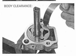
Measure the side clearance using a straight edge and feeler gauge.
