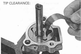
Measure the pump body clearance.
