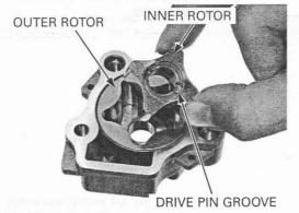
Install the oil pump shaft through the inner rotor and oil pump body.
