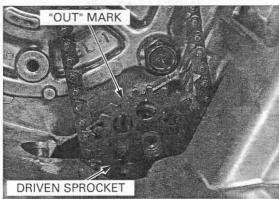
Apply a locking agent to the oil pump driven sprocket bolt threads.
