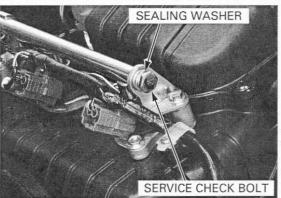
Attach the fuel pressure gauge to the fuel rail.
